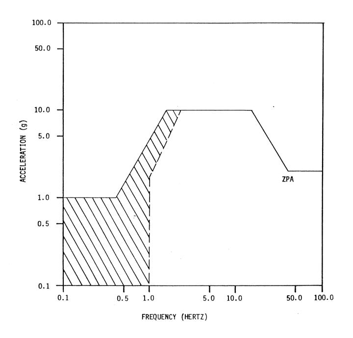
REQUIRED RESPONSE SPECTRA (RRS) FOR 2% OF CRITICAL DAMPING
